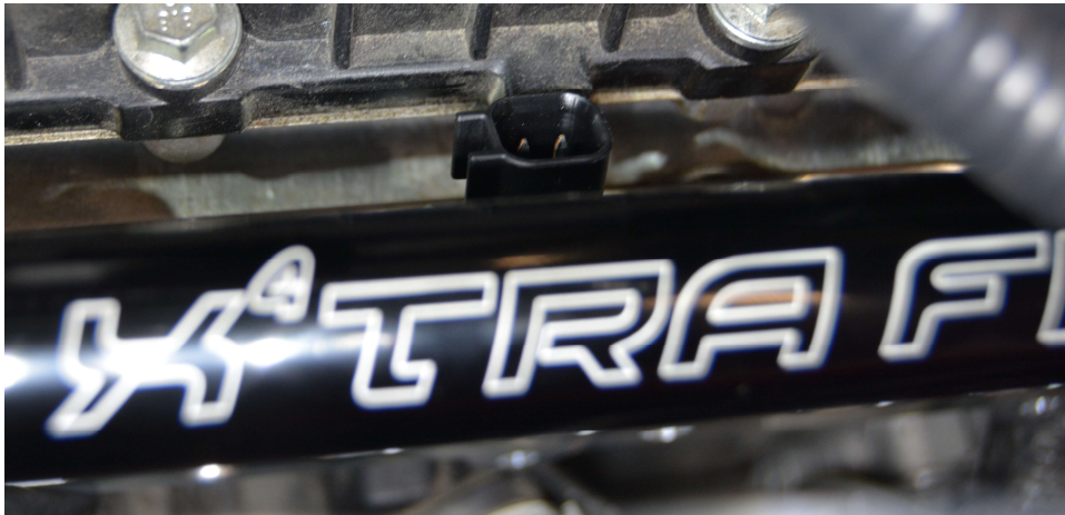
Figure 9 - Injector clearing the cut tab
