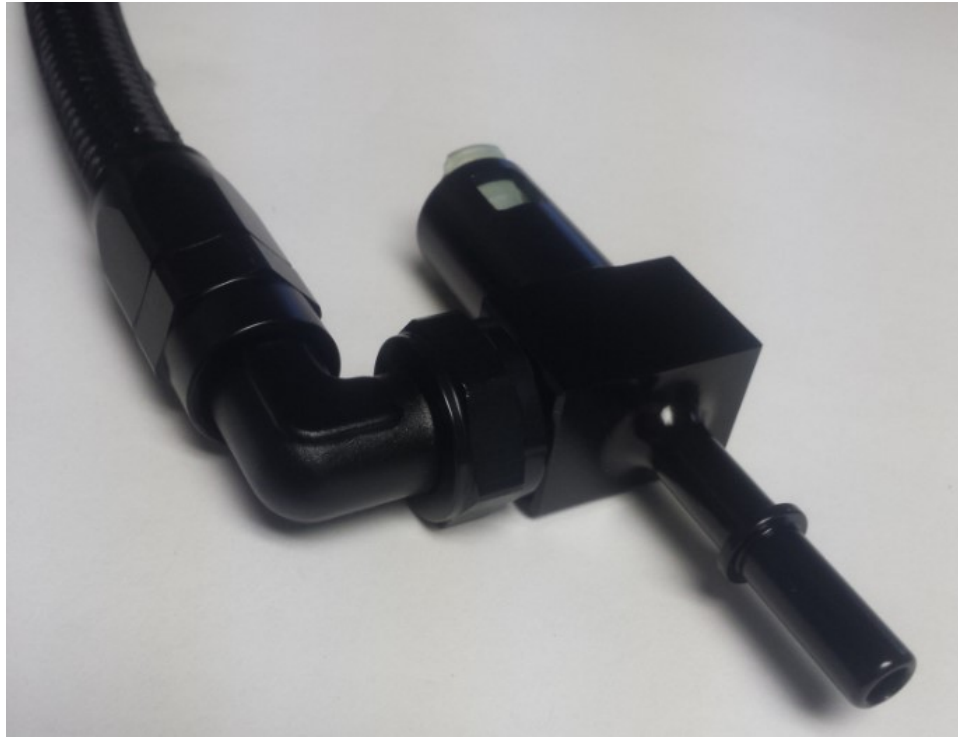
Figure 16 - Fuel Line connected to Fuel Tap
