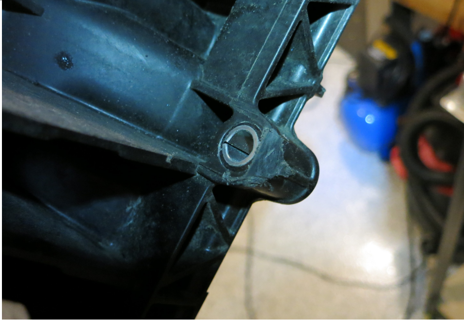
Figure 10 - Intake Manifold modified for clearance
