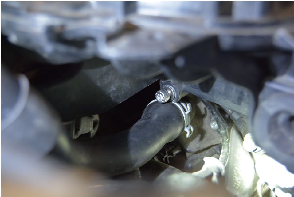
Figure 11 - Intake Manifold clearing the PCV Hose
