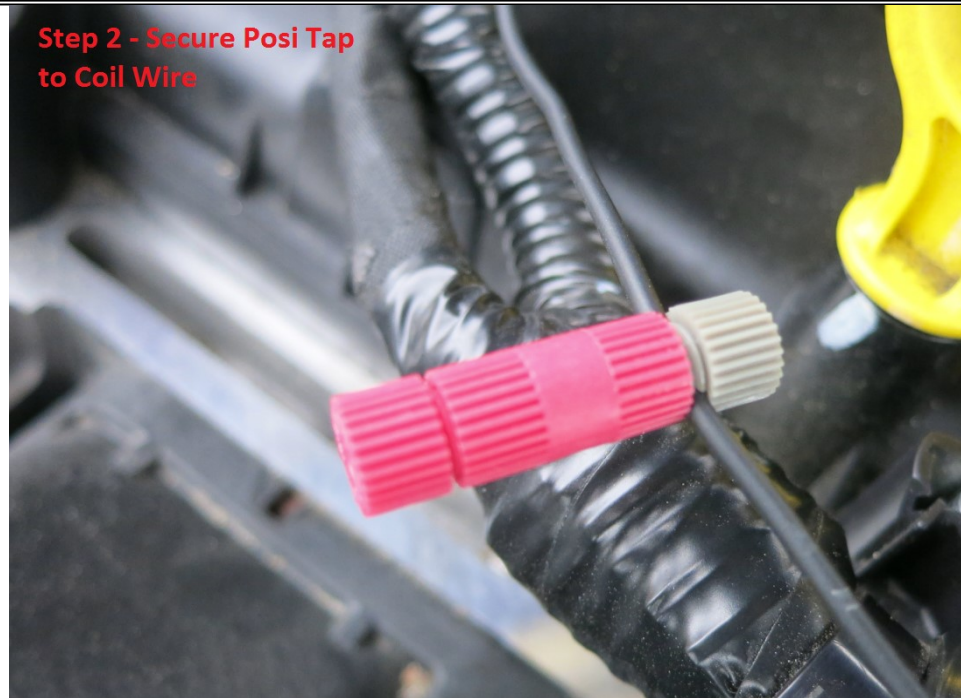
Figure 28 - Posi-Tap Instal Step 2
