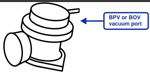
12. Gently connect and secure this hose to the BPV IN port on the GA using the provided hose clamps.
