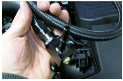
20. Disconnect the high pressure fuel pump (HPFP) feed line from behind the HPFP. It is marked by a red arrow below. This rubber flexible feed line connects to a supply hard line coming from the tank. The line is 5/16" and the best tool to use for disconnecting it is the one supplied in the kit. Select the 5/16" collar from the kit.
