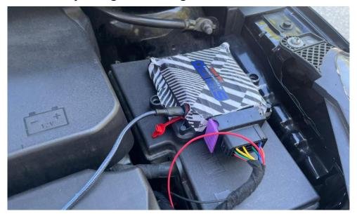
30. Now it is time to get your RPM signal connected. The wiring loom used an adapter harness to read the RPM signal directly from the cam sensor. Remove the OEM cam sensor connector, attach OEM connector to the adapter harness and connect the new grey connector to the OEM cam sensor, use zip tie to secure the connector.
