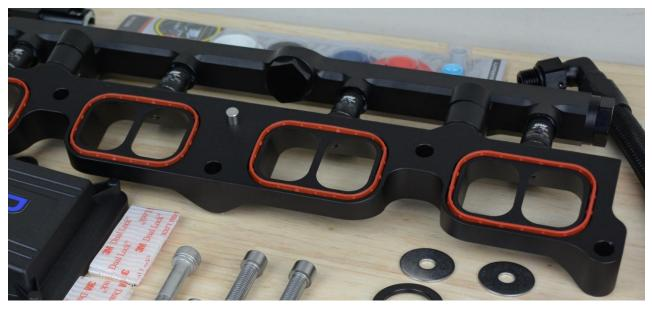
13. Mount the plate to the head using the M8 Washers and M8x40mm bolts provided. (Step 10 from radium instructions)
