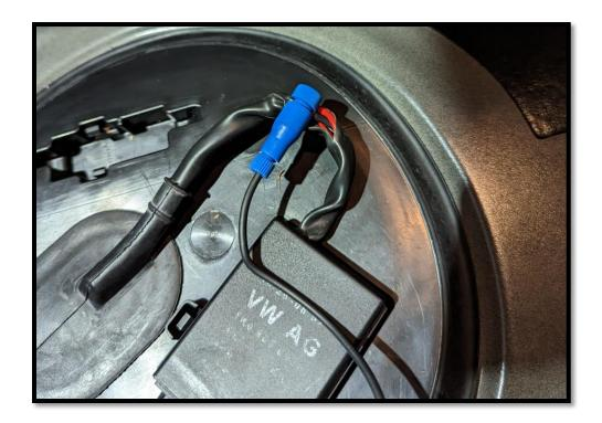
TIP: Before putting the seat cushion down, key on and listen for the pump priming. Check your fuel level display as well to make sure it is reading correctly.
