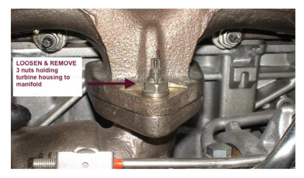
k. Remove the disconnected turbo assembly from the vehicle.
