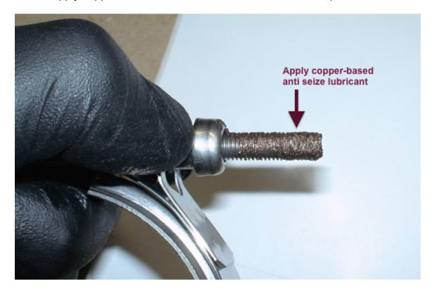
c. Position and Secure Garrett GT/GTX turbo to V-band adapter. NOTE: Please ensure v-band flanges are fully seated before tightening the V-band clamp.
