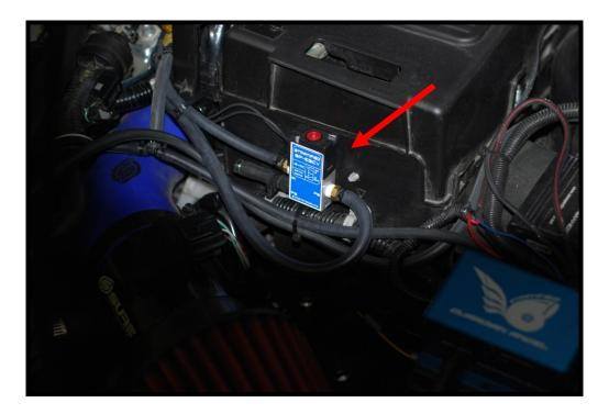
3. You will first need to located and disconnect the OEM electronic boost control solenoid electrical connector. The OEM solenoid is attached to the OEM turbocharger compressor housing. The diagram below shows the connector.
