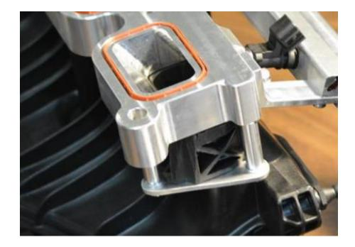
16. Place the included FoMoCo gaskets into the grooves of the Intake Spacer
