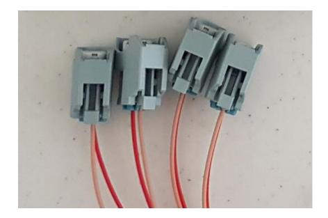
36. Now it is time to get your tach signal connected. To do this you need to tap into the **leftmost** wire for **each** of the 4 coil packs. Each tapped coil pack connects to one of the 4 **yellow/black** wires of the Aux Fuel Controller.
