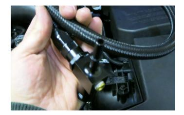
26. Disconnect the high pressure fuel pump (HPFP) feed line from behind the HPFP. It is marked by a red arrow below. This rubber flexible feed line connects to a supply hard line coming from the tank. The line is 5/16" and the best tool to use for disconnecting it is the one supplied in the kit. Select the 5/16" collar from the kit.
