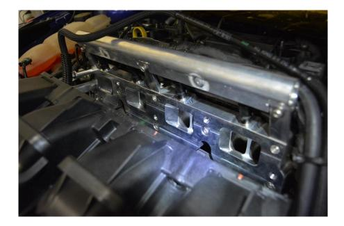
18. Make sure the injector tab is lined up with the manifold tab where the gasket shows through. This will point the electrical connectors directly behind the rail.
