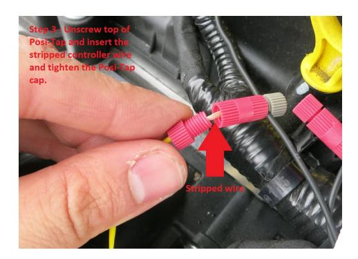
38. Now it's time to connect to the MAP sensor wire. The OEM MAP sensor wire is the leftmost on the connector. Most cars have this as gray or gray/purple. Use a Posi-Tap connector to connect this MAP sensor wire to the **green** wire on the Aux Fuel Controller.
