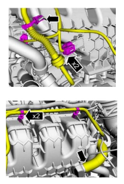
*NOTE:* The throttle body electrical connector can be a little tricky to disconnect. It might be useful to loosen the intake manifold to give yourself more clearance.
