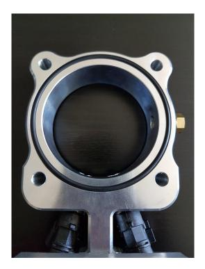
15. Carefully sandwich the throttle body spacer between the throttle body and intake manifold. The O-ring on the spacer should be facing TOWARDS the throttle body. The fuel rail should be pointing TOWARDS the driver's side.
