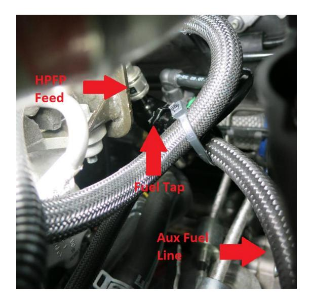
24. Secure the fuel line using the large Zip ties.
