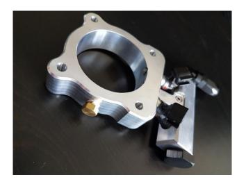
16. Install the longer throttle body bolts supplied using a 5mm hex wrench and M6 washers to hold the throttle body to the manifold and torque to 89 inch-pounds.
