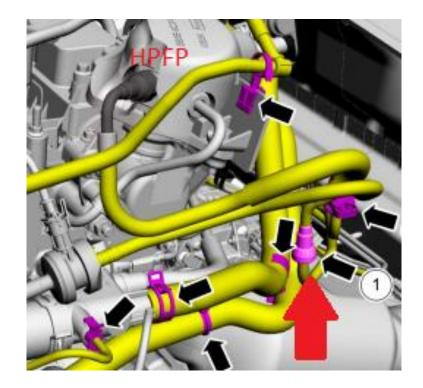
22. Place the 5/16" collar on the hard line where the arrow is pointing with the flat section away from the fuel line connector and push it between the connector and hard line. The connector should pop off without much force.
