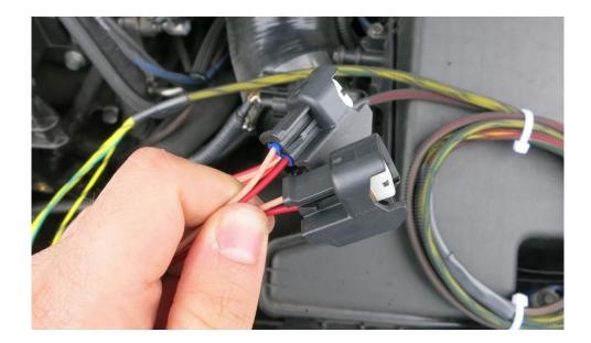
31. Now it is time to get your tach signal connected. To do this you need to tap into the **leftmost** wire for **each** of the 4 coil packs. Each tapped coil pack connects to one of the 4 **yellow/black** wires of the Aux Fuel Controller.
