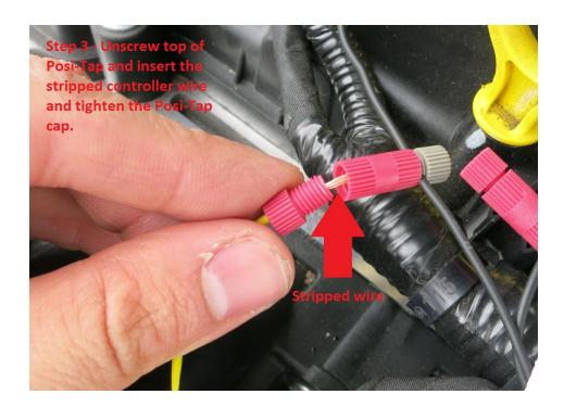
33. Now it's time to connect to the MAP sensor wire. This wire can be found right at the MAP sensor on the manifold or a little higher up the engine harness for a cleaner install. It is a **gray wire with a purple stripe**. Use a Posi-Tap connector to connect this MAP sensor wire to the **green** wire on the Aux Fuel Controller.
