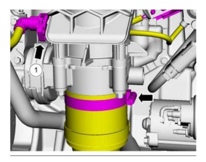
11. Disconnect the vacuum and electrical connections from the manifold and throttle body as shown below:
