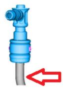
23. Place the fuel line tap on the 5/16" hard fuel supply line and re-attach the HPFP feed line to the top of the tap. Make sure all fuel connections click into place.
